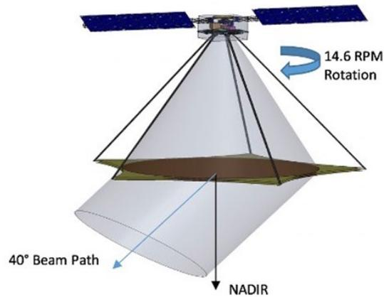
**Figure 1: Illustration of the GLOWS antenna beam steering provided by its phase-shifting meta-lens antenna.**
