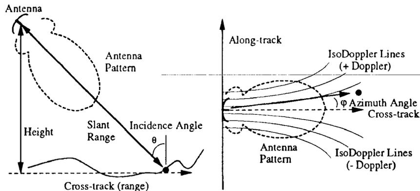
Figure 1: SAR observation geometry.
