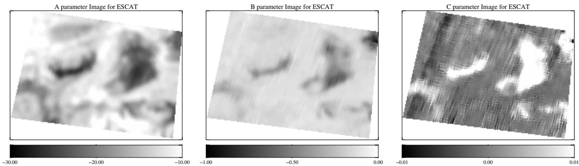
Fig. 4. Parameters of the quadratic incidence angle model fit to the ERS data over the Erg Occidental/Oriental.
