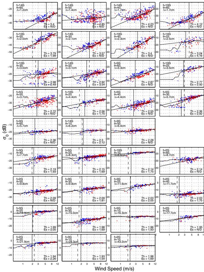
Fig. 2. H-pol YSCAT data plotted as a function of wind speed for each Bragg wavelength. The straight line through the data is the linear least-squares fit. The curved line is the non-parametric fit. The solid vertical line is the theoretical threshold wind speed (Th). The dashed line is the threshold wind speed estimated from the YSCAT data (Es).
