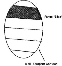
Figure 2: Fig. 2: Conceptual Diagram of Range Resolution Slice
