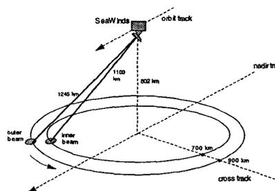
Figure 1: Fig. 1: *SeaWinds* Measurement Geometry
