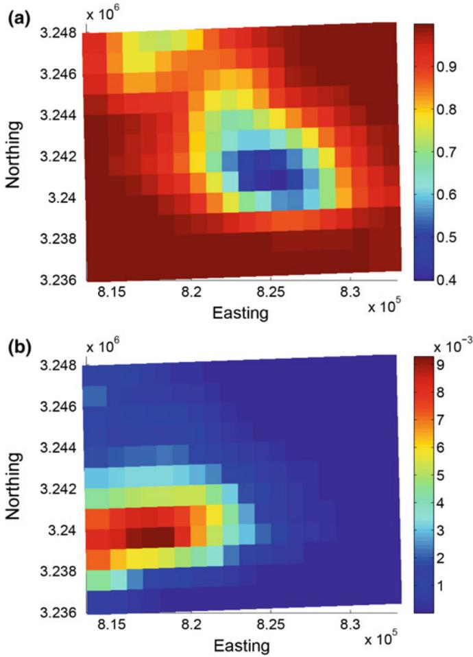
**Fig. 1.6** **a** Rain-induced atmospheric attenuation and **b** atmospheric backscatter computed from NEXRAD observations over the region in Fig. 1.4
