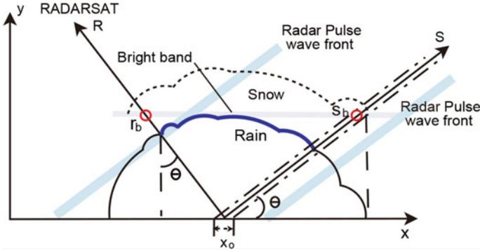
**Fig. 1.2** Schematic diagram of the SAR scattering geometry for a rain cell. The *oblique lines* represent the radar pulse under the approximation of plane wave incidence
