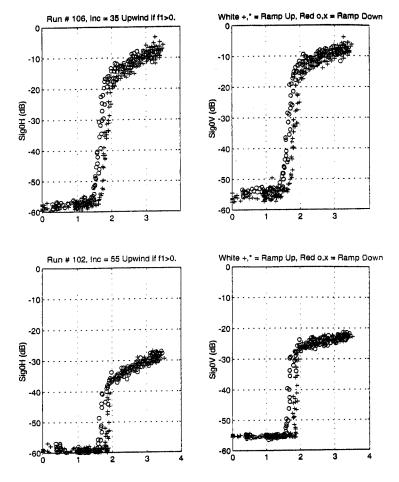
Figure E.2. Sigma-0 versus wind speed at Ku-band looking upwind. The abscissa is the mean wind speed measured at 3 cm above the mean water level. (a) Top panels: incidence angle =  $35^{\circ}$ , air temperature =  $23.8^{\circ}$  C and water temperature =  $26.7^{\circ}$  C. (b) Bottom panels: incidence angles =  $55^{\circ}$ , air temperature =  $24.0^{\circ}$  C and water temperature =  $27.8^{\circ}$  C.
