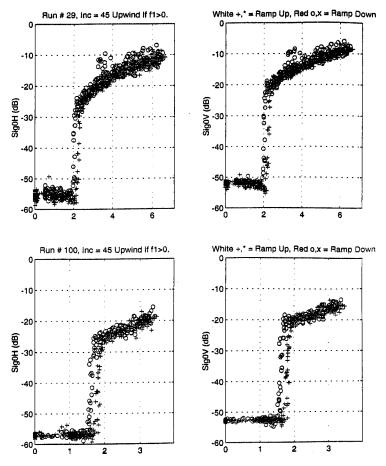
Figure E.1. Sigma-0 versus wind speed at Ku-band looking upwind at  $45^{\circ}$  incidence. The abscissa is the mean wind speed measured at 3 cm above the mean water level. (a) Top panels: air temperature =  $18^{\circ}$  C and water temperature =  $8^{\circ}$  C. (b) Bottom panels: air temperature =  $22.7^{\circ}$  C and water temperature =  $29.4^{\circ}$  C.
