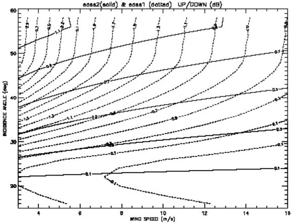
Figure 5.3. Comparison contour plot of the upwind/downwind ratio of SASS-1 and SASS-2. The ratio (in dB) is defined as the ratio of sigma-0 at  $=0^{\circ}$  to sigma-0 at  $=180^{\circ}$
