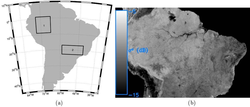
Figure 2: (a) Regions of homogeneous backscatter used in study. (b) SIR images showing backscatter. (quev-a-Ama01-257-260.sir)
