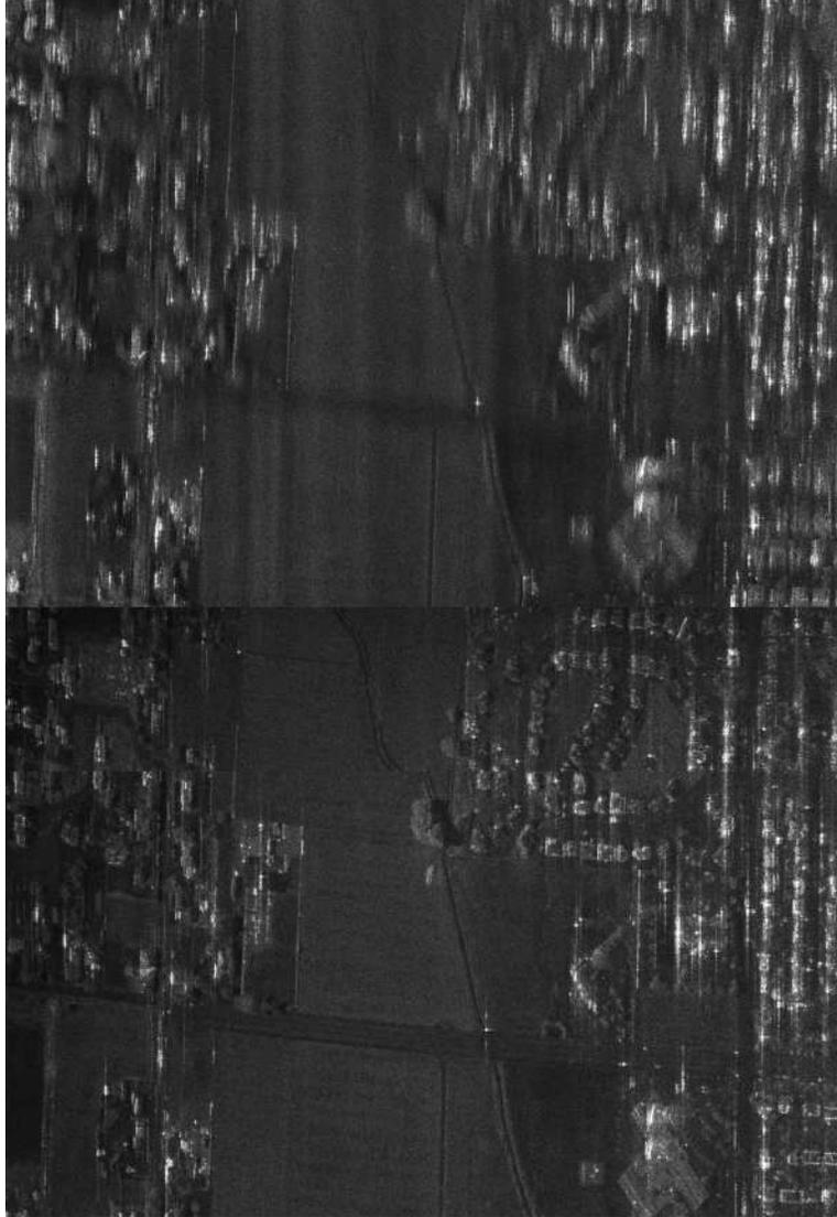
Figure A.1: Images created from NuSAR data. The top image shows the target scene without any motion compensation. The bottom image is after motion compensation has been applied. The improved focusing is apparent.
