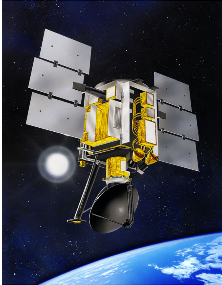
Figure 2.4: Artist's rendering of the SeaWinds instrument aboard the QuikSCAT satellite [56].
