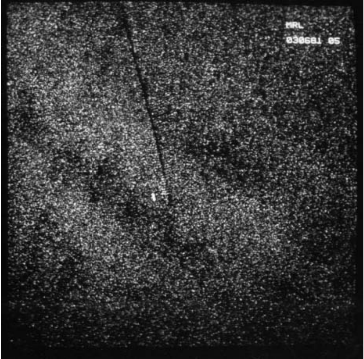
Figure 3.15: Actual SAR image of a boat moving in the cross-track direction toward the bottom of the image. The long dark line is the boat's wake, and the bright spot near the center is the boat, which is clearly mislocated from its expected position at the head of the wake. (Source: [74])
