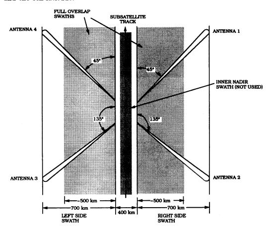
Figure 2.1: SASS antenna illumination pattern
