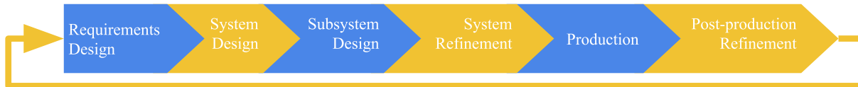
Figure 2.4: Illustration of the flow of a typical system design process [27]. Design flows in sequence from stages on the left to stages on the right. Iteration typically occurs if a next-generation product is approved after production of the first, as illustrated by the yellow, negative-feedback arrow.
