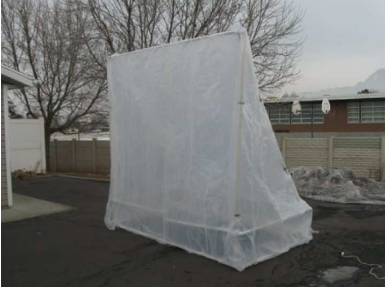
Figure 5.5: Plastic tent used to keep the scanning platform warm and to prevent binding, with its PVC frame visible through the greenhouse plastic.
