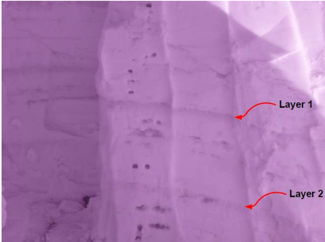
Figure 6.16: Infrared image (wavelengths around 930 nm) of the lower two-thirds of the snowpack during the first deployment. Two layers of dangerous faceted snow appear as dark, 4 cm bands across the snowpack.
