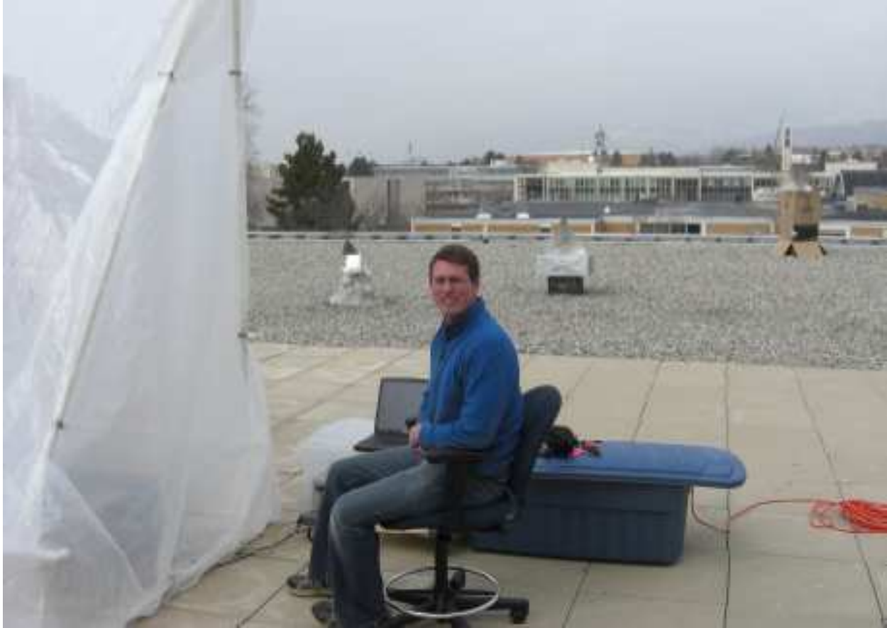
Figure 6.1: Range set up on the roof of the engineering building with corner-reflector Targets #1 through #3 positioned from left to right. The scanning platform is in the plastic tent in the foreground.
