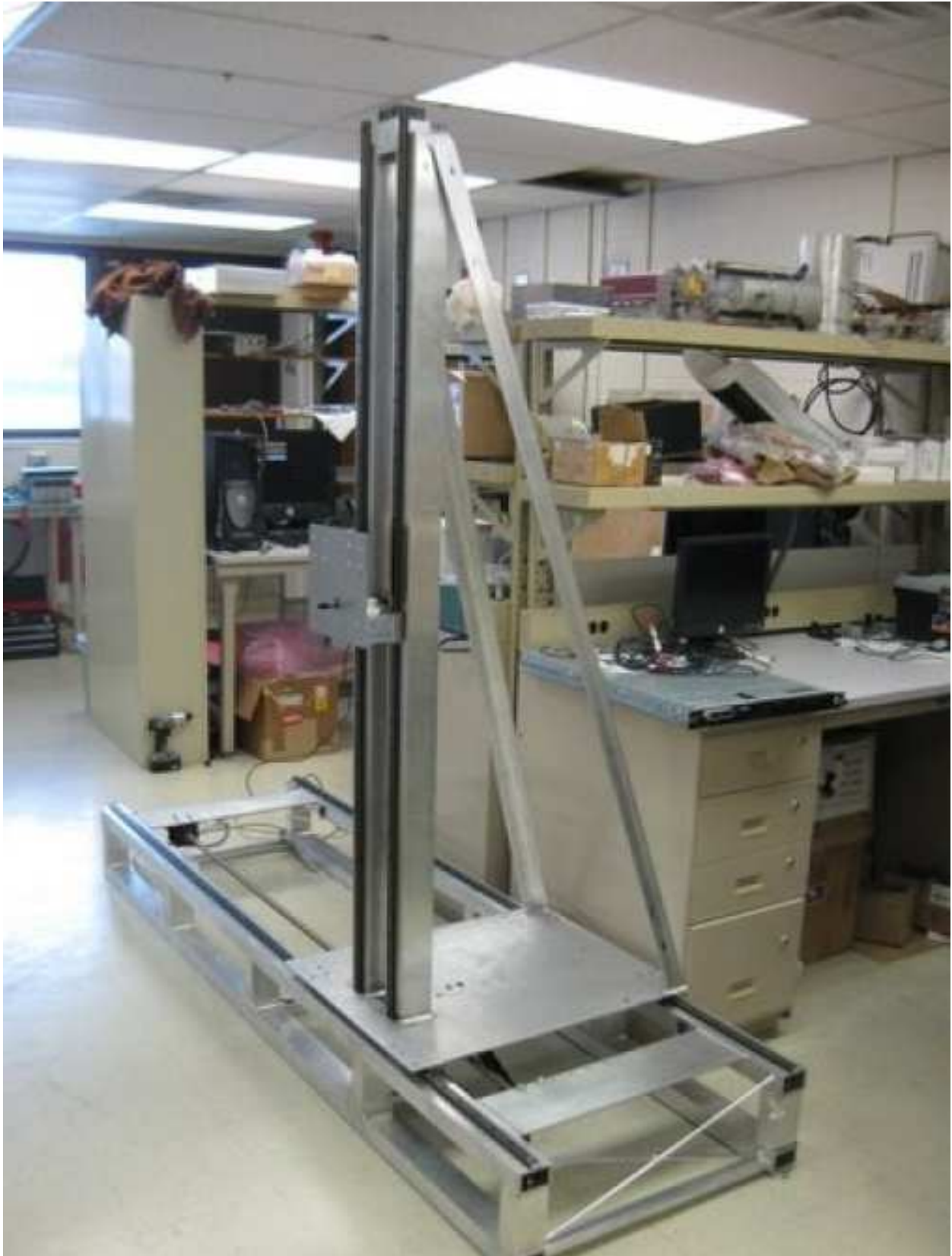
Figure 5.4: Side view, allowing the completed scanning platform to be viewed in its entirety. The screw used to translate the base plate horizontally is visible within the box of the horizontal component. The driving motor for the horizontal component is attached on the far end.
