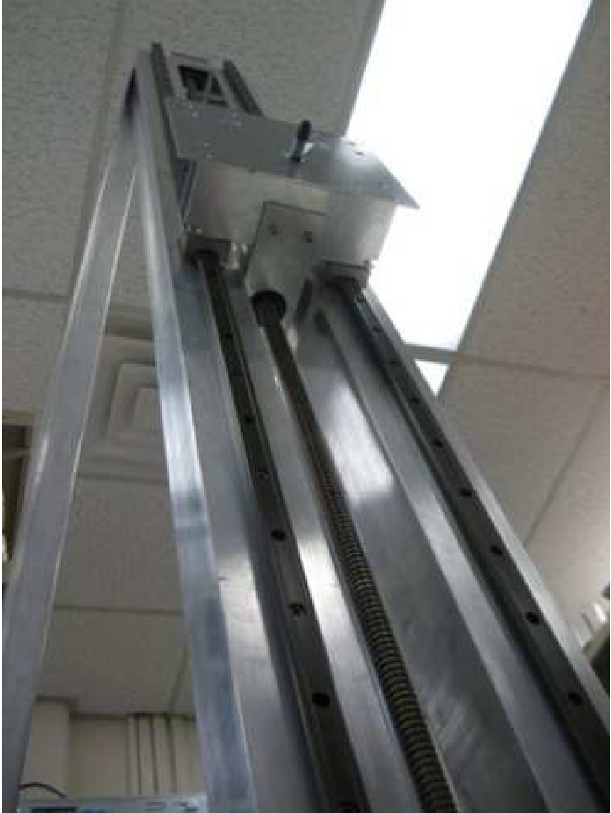
Figure 5.3: Picture of the vertical component of the completed scanning platform with an antenna mount and the driving screw visible.
