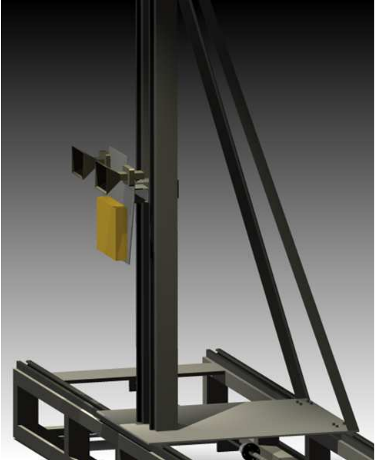
Figure 5.2: Drawing of design for a ground-based platform generated in AUTOCAD, demonstrating the inverted T-shape design that allows motion along the horizontal component extending out of the picture and along the vertical component. The rendering also depicts the horn antennas on the antenna-mount plate disposed more than half way up the vertical component with the bronze-colored microASAR module, discussed below, positioned underneath.
