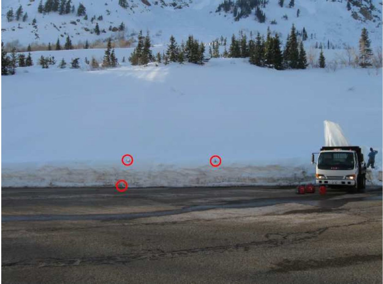
Figure 6.17: Side view of the second deployment, picturing the snowpack and the relative orientation of the scanning platform during the second deployment. Three corner reflectors used to verify the location of snowpack are circled in red, with the ranges to those corner reflectors provided in Table 6.5. The man just behind the truck is taking pictures of a snow pit from which measurements of snowpack layers are made in an effort to correlate physical measurements with radar data. A snow pit adjacent to the one in the picture was dug for the first deployment.
