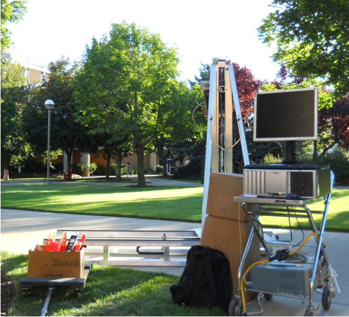
Figure 5.1: Photo of the scanner in operation with accompanying equipment. Normally a laptop computer is used rather than the desktop shown here. (Experiment 2)
