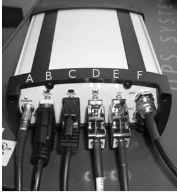
Figure 3.2: Connections of the NovAtel: A) Power Socket B) To MOTRON C) To SAR System D)&E) To IMU F) To Antenna
