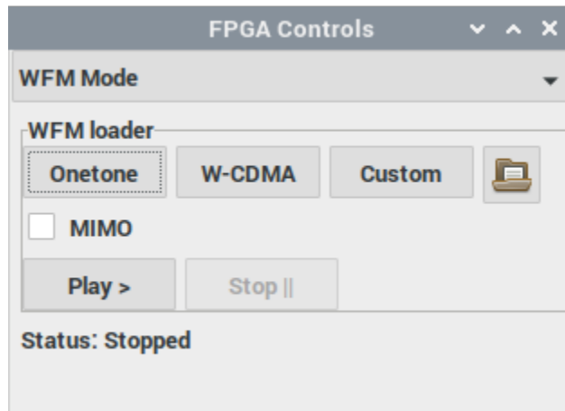
Figure 4.10: LimeSuite GUI FPGA controls dialog window used to feed data into the transmit portion of the SDR.
