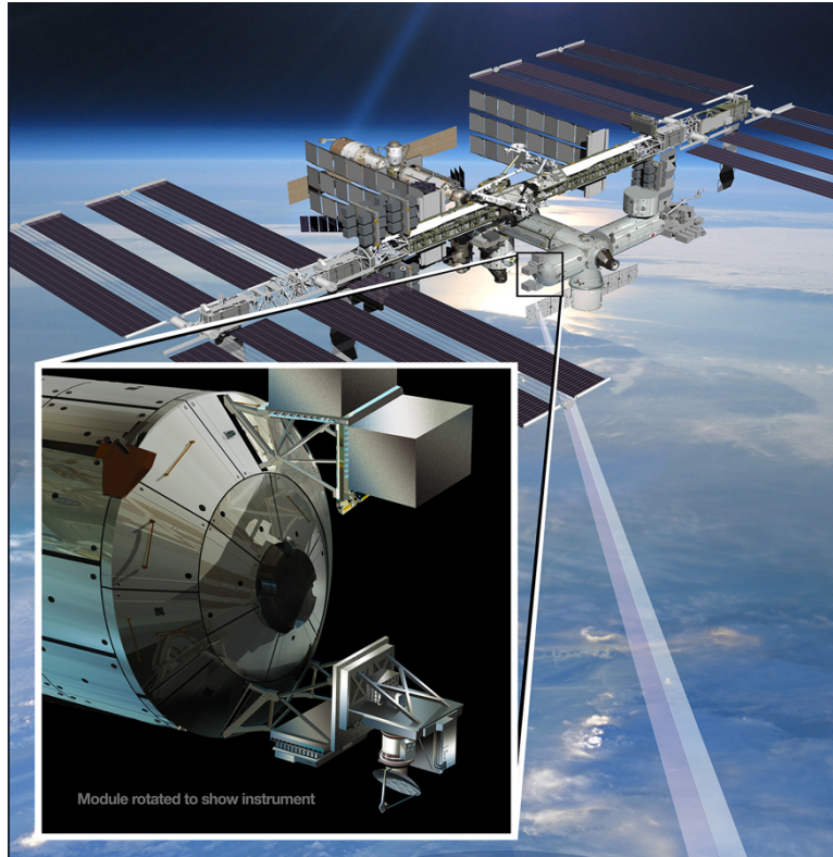
Figure 2.7: The RapidScat scatterometer on the Columbus module of the International Space Station (ISS). RapidScat was launched to replace the QuikSCAT mission. Image courtesy of NASA [7].
