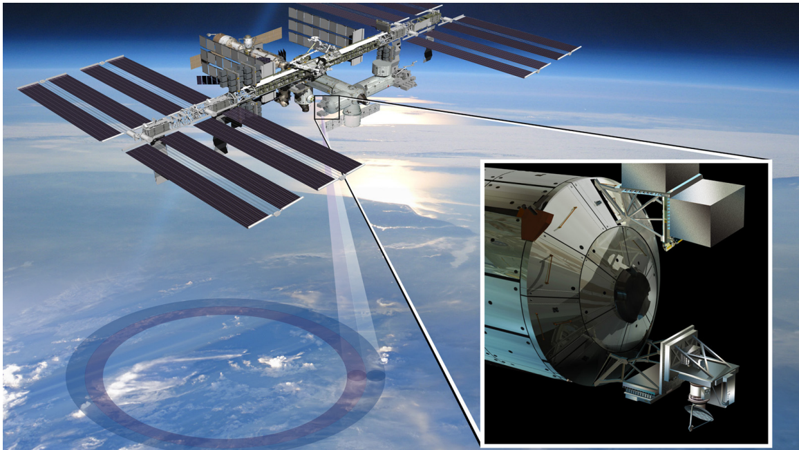
Figure 1.5: Artist's rendering of the RapidScat scatterometer on the Columbus module of the International Space Station (ISS). From JPL's RapidScat Mission website [7].
