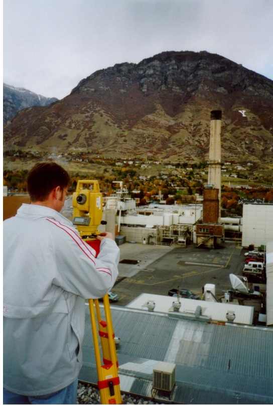
Figure A.2: Nick Williams, a BYU Civil Engineering Student, surveys Y Mountain to measure the elevation angle of its summit.
