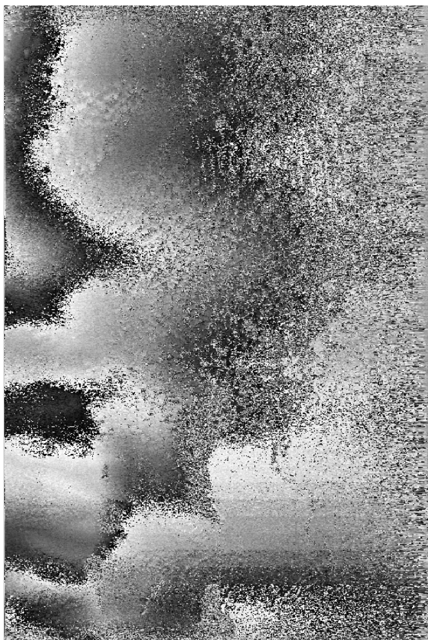
Figure 4.11: A phase wrapped motion compensated interferogram from pass 1124 over Wolf Creek, UT. Note that by compensating both channels to a single track, the a flat earth differential phase is removed – i.e. there are less phase fringes.
