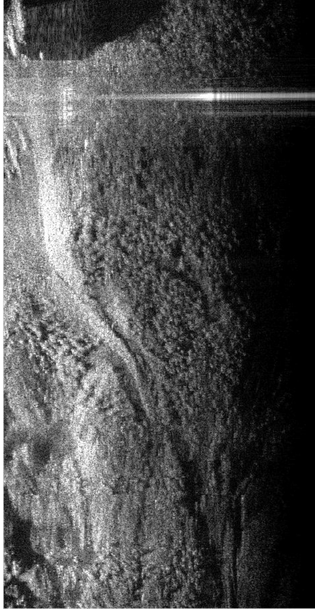
Figure 4.8: Flight U, pass 2209 over the Slungullion slide with Narrowbeam motion compensation applied using a segmented ideal track.
