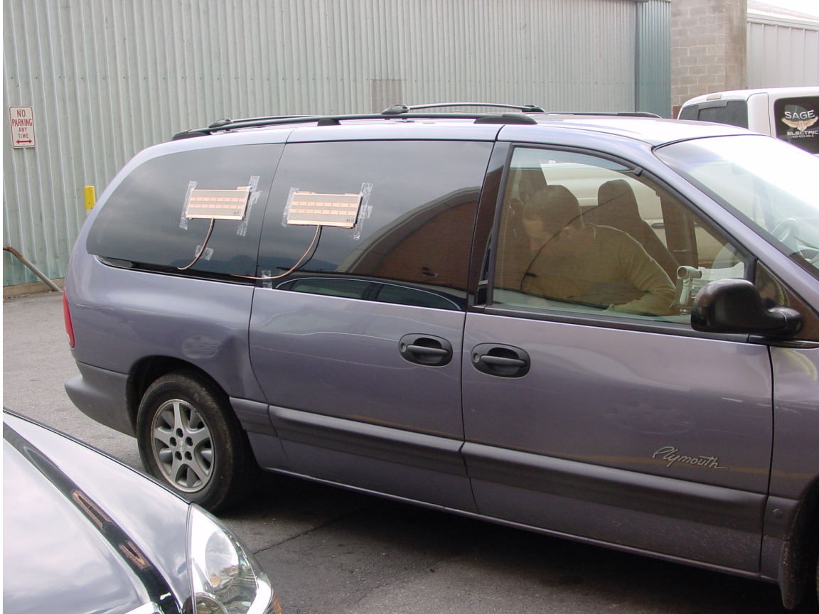
Figure 4.6: Photograph of the \mu SAR test setup with antennas mounted to the side of a van.
