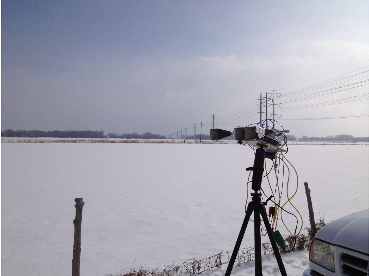
Figure 5.4: Front view of the data collection radar sitting on a tripod. The high gain horn antennas can be seen at the front of the radar.
