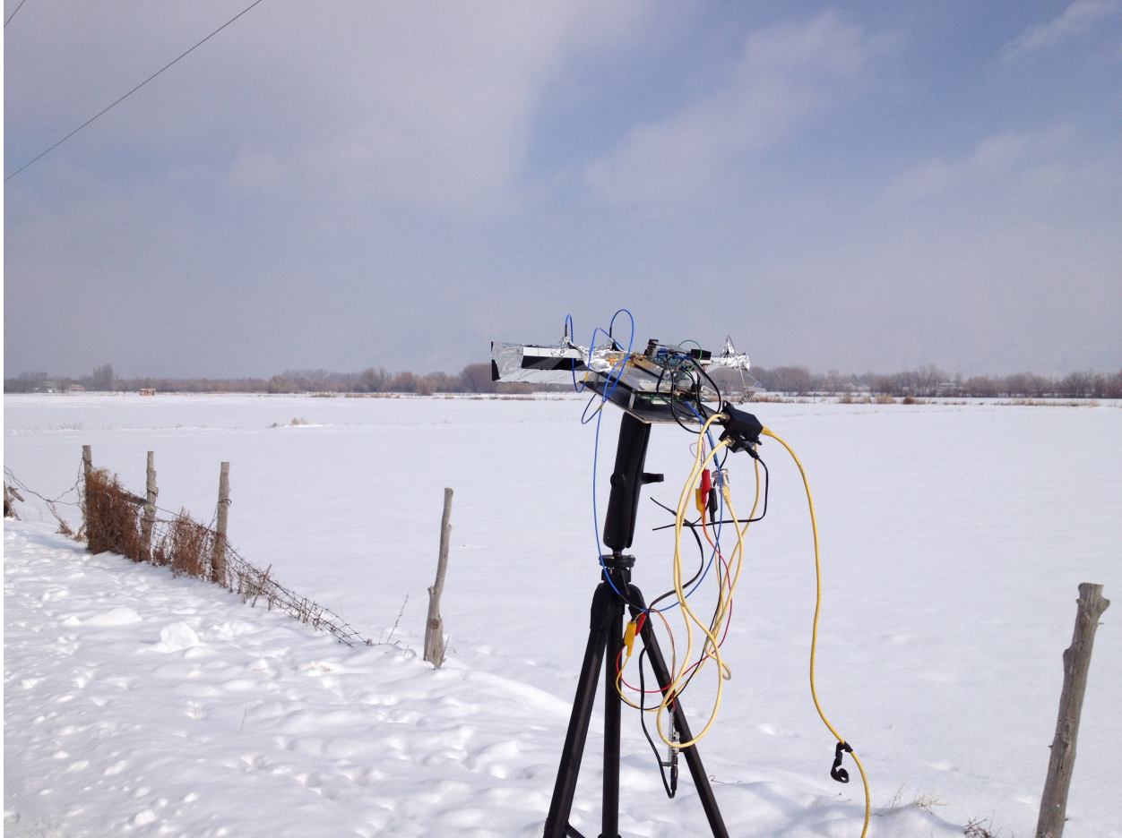
Figure 5.3: Back view of the data collection radar sitting on a tripod showing many of the coaxial and power cables required to run the system.
