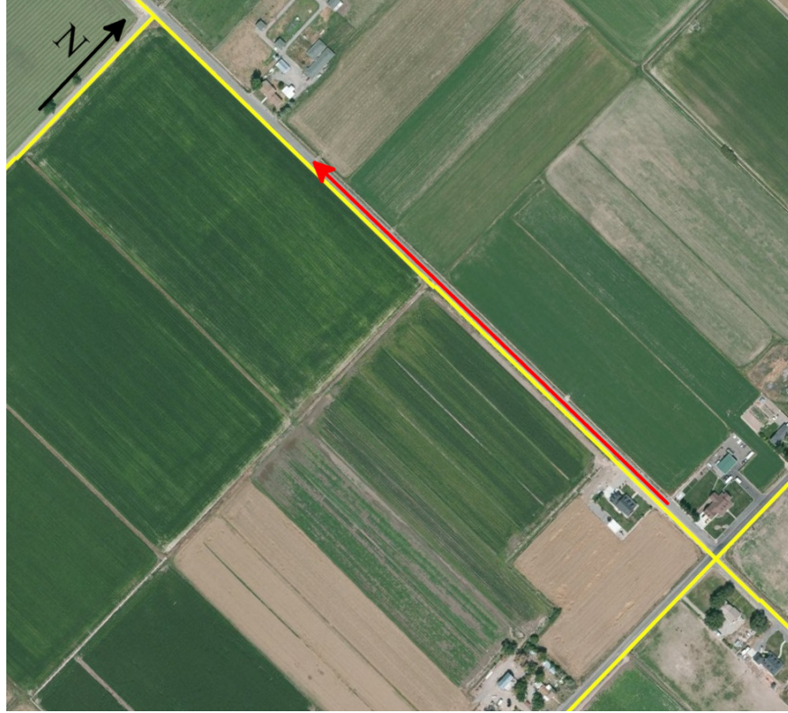
Figure 5.3: Shapefile representing the area depicted in Fig. 5.2. The roads in the image are highlighted in yellow. The red arrow indicates the target’s path during the SAR collection. Since we can get the gps coordinates of the start and ending points of the target’s path from the shapefile, we can easily calculate the road’s heading by using Eq. (5.1).
