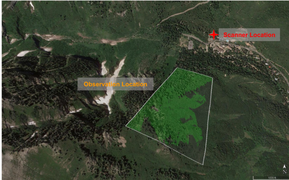
Figure 3.10: The scanner and observation locations. The radars viewshed is highlighted in bright green while the white trapezoid highlights the coverage area within the beamwidth. The intersection of these two areas represents the observable area.
