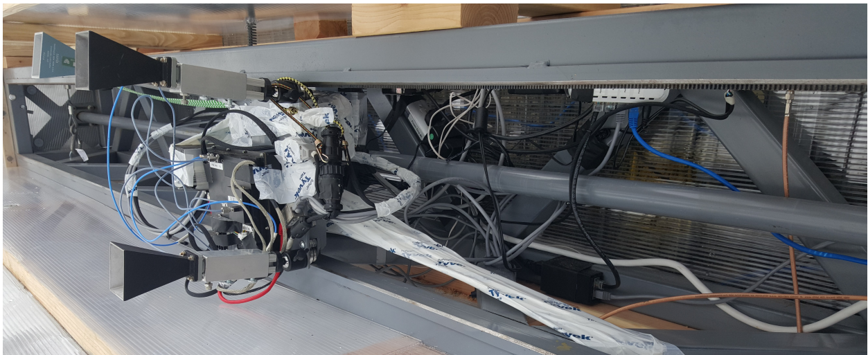
Figure 3.6: Image of antennas and radar on the gantry mounted sled, all residing on the scanner gantry. Assorted RF, Ethernet, and power cables also shown.
