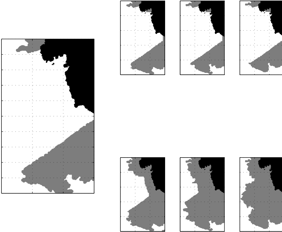
Figure 3.11: Simulated recovery capability of modified versus original RL algorithm for a sequence in western Antarctic. Gray represents ice, white represents ocean, and black represents land. The left-most image (JD 1) was generated from data with a missing satellite swath. The top sequence shows JD 3-5 from the original RL algorithm, and the bottom sequence shows JD 3-5 from the modified algorithm. (JD 2 is skipped because of a complete lack of data).
