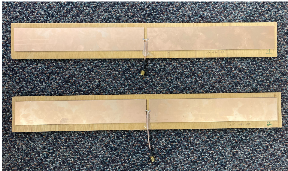
Figure 3.10: The constructed strip dipole models, where Antenna 1 is on the top and Antenna 2 is on the bottom.
