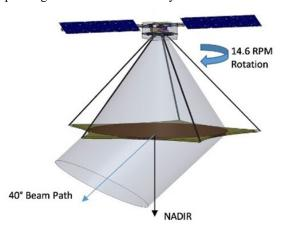
Figure 1: Illustration of the GLOWS antenna beam steering provided by its phase-shifting meta-lens antenna.
