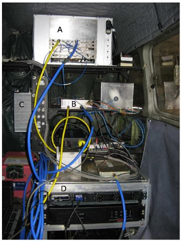
Figure 1. Equipment setup inside testbed aircraft. Labelled are: (A) pulsed SAR system, (B) CW microASAR system, (C) BYU Motron, and (D) computer for data storage and processing. The configuration shown can be rearranged to accommodate new systems for testing.
