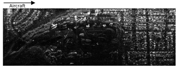
Figure 3. Stripmap SAR image of a portion of Brigham City, UT processed from data gathered using microASAR on the Surf Angel testbed. The suburban area is interrupted by a gravel pit in the center of the image which is much less reflective.
