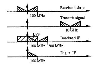
Figure 3: BYU SAR signal frequency plan.
