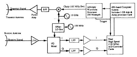
Figure 2: BYU SAR block diagram.
