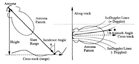
Figure 1: SAR observation geometry.
