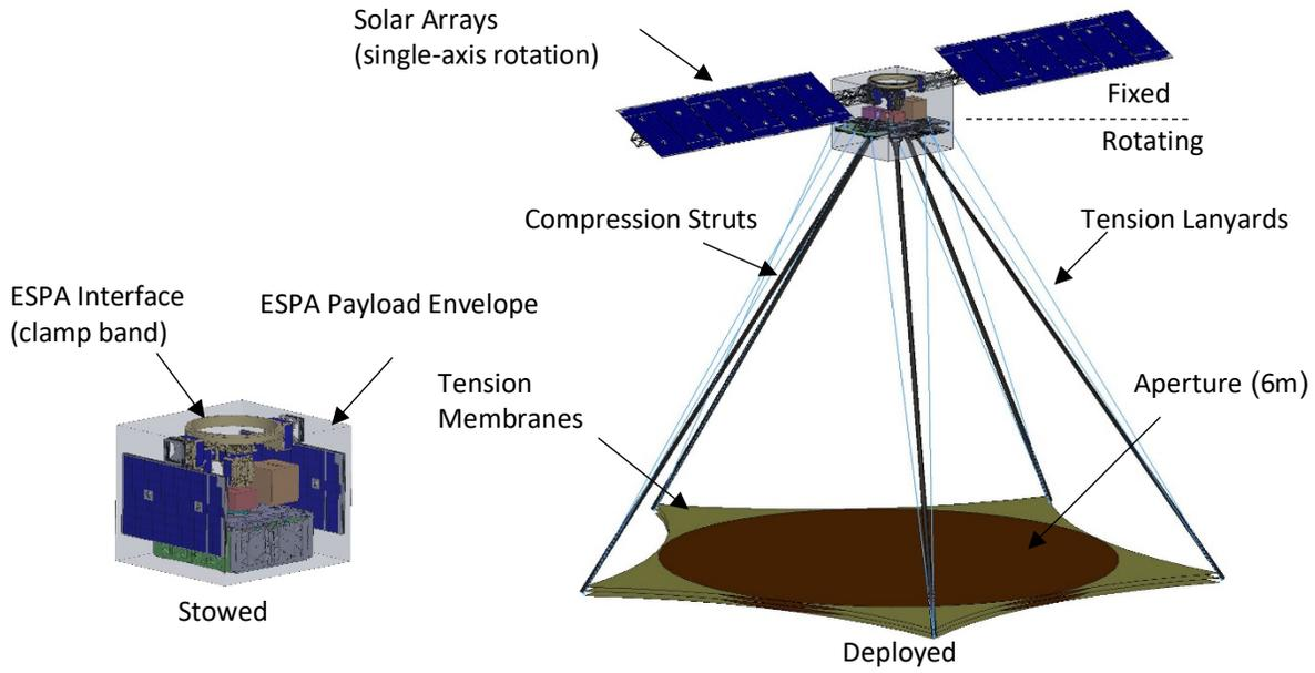
Figure 2. Illustration of the GLOWS launch and deployed configurations.
