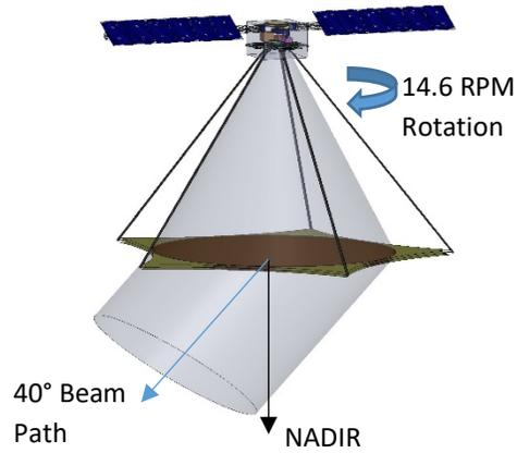
Figure 3. Illustration of the GLOWS antenna beam steering provided by its phase-shifting lens antenna.
