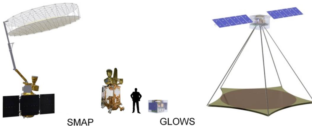
Figure 1. Comparison of SMAP and GLOWS integrated in an ESPA-class spacecraft. Note the similarity of deployed configurations and the contrast of launch configurations.
