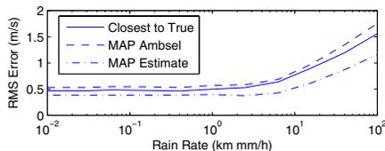
Fig. 2. RMS error versus rain rate for ideal ambiguity selection, MAP ambiguity selection, and MAP estimation.
