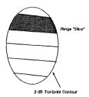
Figure 2: Fig. 2: Conceptual Diagram of Range Resolution Slice
