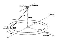
Figure 1: Fig. 1: SeaWinds Measurement Geometry
