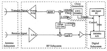
Figure 1: YSAR Block Diagram
