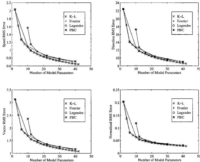
**Figure 1:** Average speed, direction, vector, and normalized rms error as a function of number of model parameters. These errors represent the difference between the nudged wind field,  $\mathbf{W}$ , and the least-squares model fit,  $\hat{\mathbf{W}}$ .
