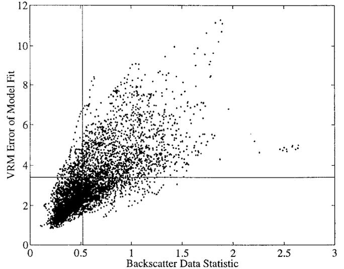
**Figure 2:** In general a field that is poorly fit by a 2 parameter KL model has a large value of the statistic,  $y$ , defined for the BC algorithm as the standard deviation of the normalized backscatter.
