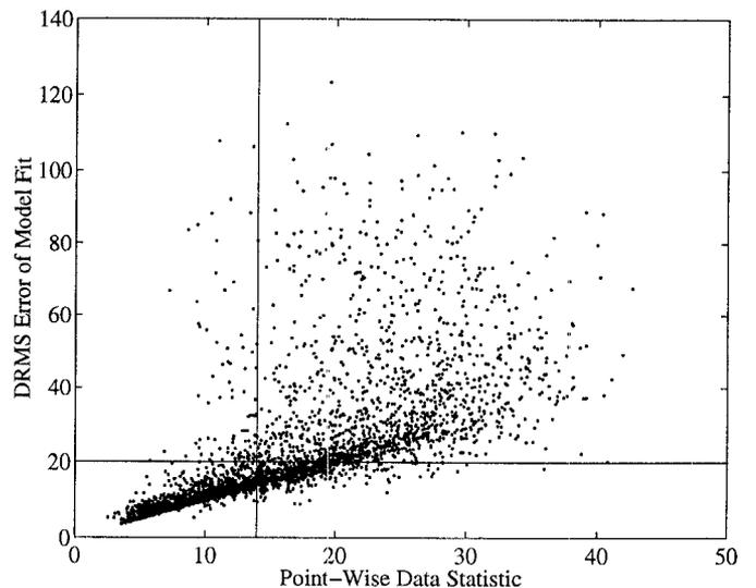
**Figure 3:** The DRMS error in a 2 parameter KL model fit to NSCAT JPL nudged wind fields is highly correlated with the PC algorithm statistic,  $y$ .
