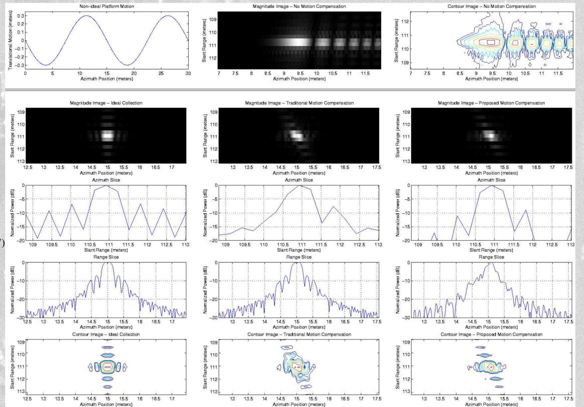
Figure 1: Simulated SAR data of a single point target with motion. The first column shows a collection without motion, the top row shows the motion and the image without compensation, the middle column shows the results of traditional motion compensation, and the rightmost column shows the proposed motion compensation.
