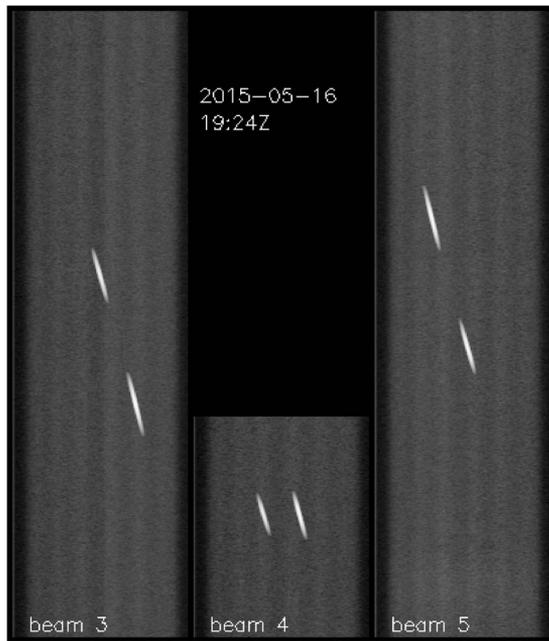
Fig. 9. Example image of the ASCAT calibration mode data showing two transponders in the right three beams. For each beam, the horizontal axis is range (cross-track), and the vertical axis is time (along-track).
