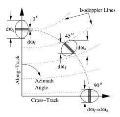
Fig. 6. Illustration of the effect antenna rotation has on the Doppler bandwidth of antenna footprint and range-resolved measurements. At  $0^{\circ}$ , the bandwidth of an antenna footprint  $(\mathrm{d}\omega_a)$  measurement is maximum, and a range-resolved  $(\mathrm{d}\omega_f)$  measurement is minimal. At  $90^{\circ}$ , the bandwidth of both measurements are equal.
