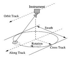
Fig. 3. Geometry of a conically scanning pencil-beam spaceborne scatterometer [7].
