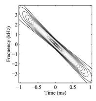
Fig. 4. Radar ambiguity function for a single LFM pulse with a down chirp.
