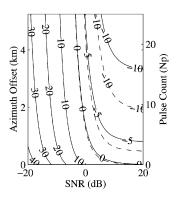
Fig. 7. Contour plot of normalized variance  $(K_p^2)$  as a function of SNR and azimuth offset and pulse count in decibels  $(20\log_{10}K_p)$  for HYDROS at  $90^\circ$  azimuth angle. The right axis is the number of pulses included in the variance sum (58), while the left axis is the corresponding azimuth distance (in km). The solid lines represent the variance for HYDROS pulses, the dashed lines represent measurement variance if the pulses were independent.
