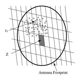
Fig. 1. Simplified geometry of a scatterometer footprint. Each  $z_i$  represents an individual scatterer. Z is the total voltage response of one resolution element, consisting of a large number of individual scatterers. The elliptical footprint is the 3-dB contour of the illumination pattern.
