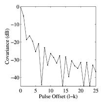
Fig. 5. Plot of  $\bar{V}_{kl}^a$  at 90° azimuth as a function of l-k for the HYDROS instrument. The figure shows that consecutive pulses have a covariance of 0.30, and pulses offset by more than two pulses are essentially independent.
