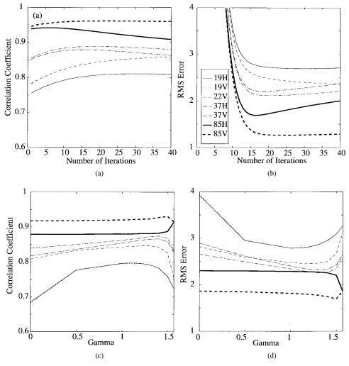
Fig. 3. Correlation coefficient and rms error between simulation results and true simulation images. (a) SIR 19-V correlation versus SIR iteration number k, (b) SIR 19-V rms error versus SIR iteration number k, (c) BGI 37-V correlation versus BGI  $\gamma$  coefficient, and (d) BGI 37-V rms error versus BGI  $\gamma$  coefficient. The 19-H and 19-V lines overlay each other.
