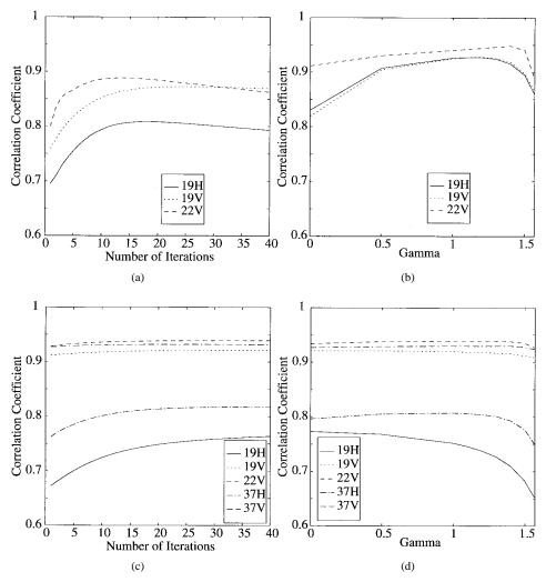
Fig. 6. Correlation coefficient between Amazon River Delta region results and nonenhanced images: (a) SIR 19 V and nonenhanced 37 V versus SIR iteration number k, (b) BGI 19 V and nonenhanced 37 V versus BGI  $\gamma$  coefficient, (c) SIR 19 V and nonenhanced 85 V versus SIR iteration number k, and (d) BGI 19 V and nonenhanced 85 V versus BGI  $\gamma$  coefficient.
