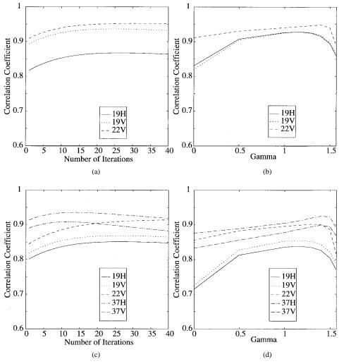
Fig. 4. Correlation coefficient between simulation results and nonenhanced images. (a) SIR 19 V and nonenhanced 37 V versus SIR iteration number k, (b) BGI 19 V and nonenhanced 37 V versus BGI  $\gamma$  coefficient, (c) SIR 19 V and nonenhanced 85 V versus SIR iteration number k, and (d) BGI 19 V and nonenhanced 37 V versus BGI  $\gamma$  coefficient.
