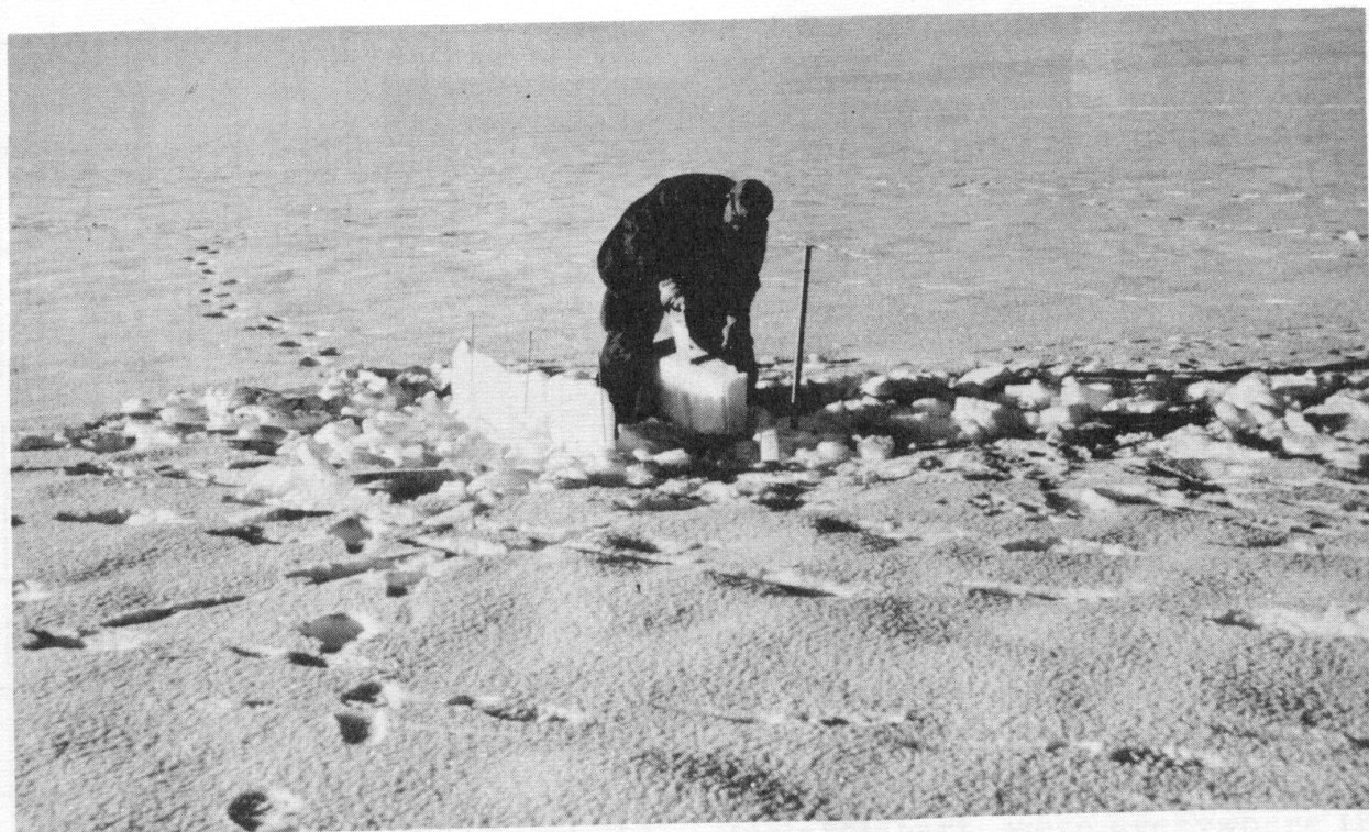
Figure 14. Frozen melt crust at station 2-70, 15 July 1954. The melt crust was 3 to 4 cm thick and resulted from the mid-July heat wave (Fig. 12). The depressions spaced about 1 to 2 m apart probably form over large ice glands such as illustrated in Figure 10b. The spacing of the large ice glands is about the same as the spacing between depressions. The glands and depressions both formed during 11 - 15 July 1954 (see p. 22).
