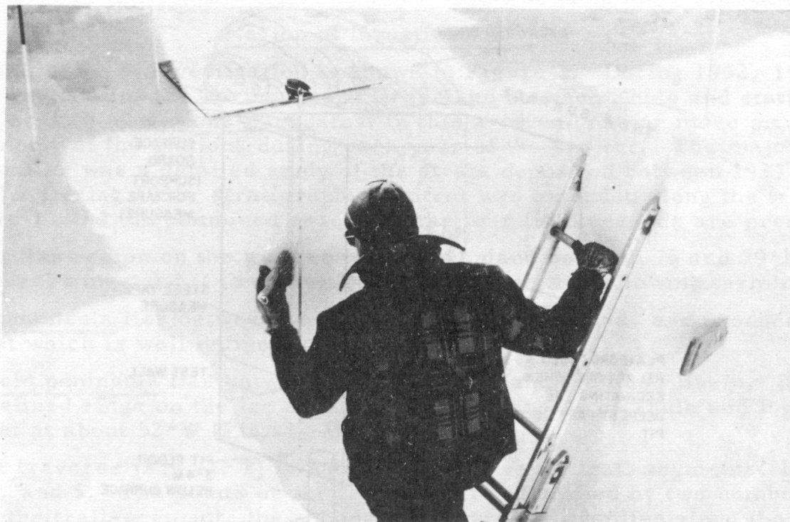
Figure 4a. Brushing test wall of pit to make strata stand out clearly in the upper 6 m, where resistance to this "erosion" varies markedly. Note undisturbed surface at edge of test wall.
